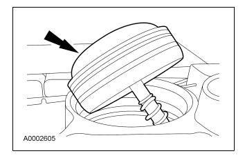
39. Using the special tool, install the retaining ring.
